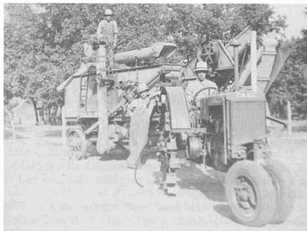
1937—Raymond, Harold and Ralph Ries at threshing time. Wheels on tractor were skeleton wheels, 2-inch wheel with off-set lugs.
